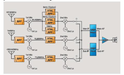
Icom's basic idea about the best receiver circuit is to reproduce high fidelity audio without internal distortion. Our answer to achieve this goal is to adopt a double conversion superheterodyne system\*. The double conversion system simplifies the electronic circuitry and reduces the number of components which cause internal distortion. The digital signal processing (DSP) technologies and image rejection mixer make it possible to adopt this system.
