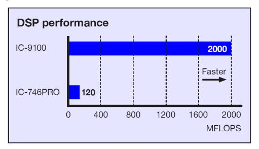
The IC-9100 employs a much higher speed DSP unit compared to the IC-746PRO/7400's DSP unit.
