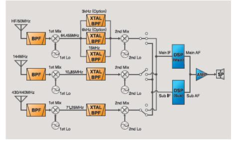
3 independent receiver circuits from the antenna connector to the second IF mixer (image rejection mixer). One for HF/6m, 2m, and 70cm. Simple receiver design reduce the number of IF stages in a receiver reduces the image and internal noise insertion points.
