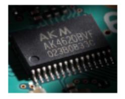
Employing the ADSP-21369 (DSP) and AK4620 (AD/DA) to provide a powerhouse of DSP performance in a HF/6m/ 2m/70cm Rig.
