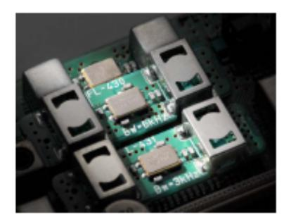
The IC-9100 comes with a built-in 15kHz 1st IF filter and can accept up to two optional filters (3kHz FL-431 and 6kHz FL-430).
