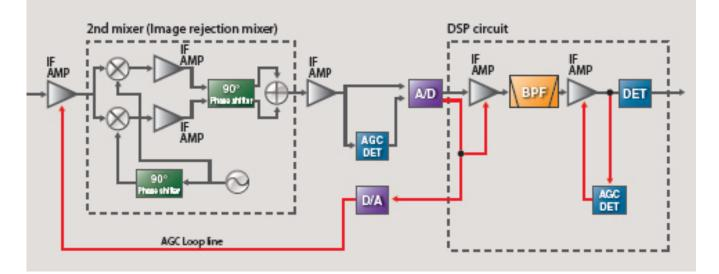
Digital IF filters, manual notch filter and other digital functions are incorporated in the AGC loop management controlled by the DSP unit. The AGC effectively works for the desired signal and rejects blocking by strong adjacent signals out of the filter passband. The AGC time constant presets (slow, medium and fast) give the flexibility and speed needed for working pile-ups. (HF/6m/2m/70/23cm\*)
