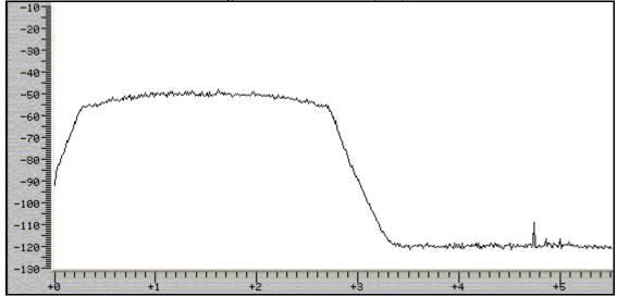
Figure 3: 500 Hz CW filter (Sharp, BPF)
