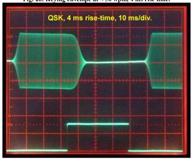
31b. CW QSK recovery test: This test was devised to address Yahoo! Group reports that CW QSK (full break-in) does not work well when using the internal keyer at speeds > 12 wpm. If a string of dits is transmitted at speeds > 12 wpm, the receiver does not recover between dits.
