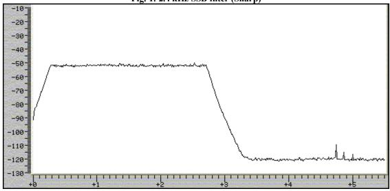
Fig. 2: 2.4 kHz SSB filter (Soft)
