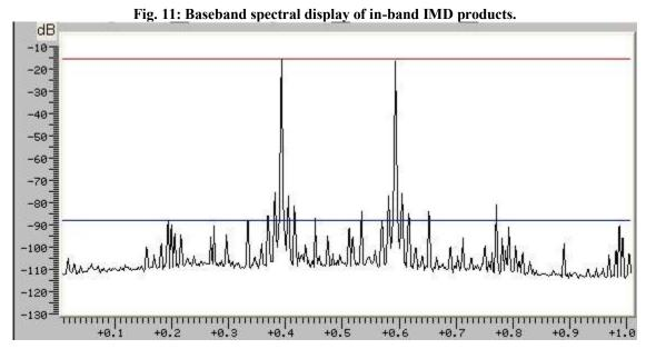
On the X-axis,  $+0.0 \text{ kHz} \stackrel{\wedge}{\_} 9999.6 \text{ kHz}$  (virtual carrier).  $f_1$  is at +0.4 kHz,  $f_2$  at +0.6 kHz. The 3<sup>rd</sup>-order IMD products are at +0.2 and +0.8 kHz respectively.
