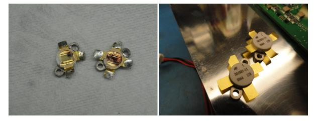
The second photo shows a small turn-up I put on the new FETs so that they are easier to remove if / when this failure happens again!
