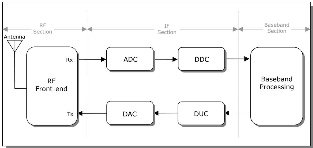
**Figure 1:** Block diagram of a generic digital transceiver
