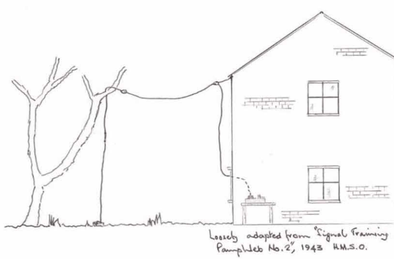
Fig.5. An end-fed inverted-L antenna, typical of some that may have been used
