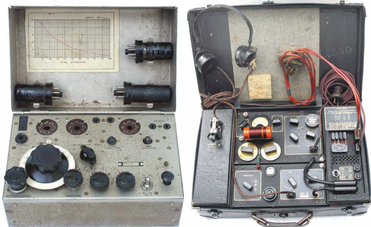
Fig. 1. The Paraset and B2 transmitter/receivers (photos by courtesy of Louis Meulstee)
